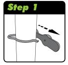
Slide the hole of the cap end without the tab over the first exposed point of the clip and push down. Stretch the tab across.
