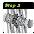
Strike the clip through the nettina/shade cloth onto the scaffolding/fencing as per normal operation.
