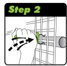
In a single action, firmly strike the KwikAz clip through the containment screening and around the pole/standard. Ensure the clip is perpedicular to the standard or ledger, and not at an angle.
